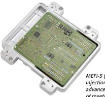
MEFI-5 (Marine Electronic Fuel Injection - Fifth-Generation), is an advanced engine controller capable of meeting all the emissions, OBD-M and driveability requirements of marine applications.
