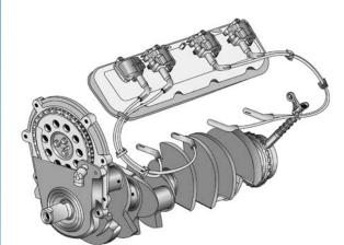
The coil-near-plug ignition system, with both crankshaft sensor and camshaft sensor, is another example of GM Powertrain bringing advanced automotive technology to the marine engine market.
